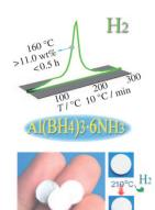
Al(BH<sub>4</sub>)<sub>3</sub>·6 NH<sub>3</sub> has been prepared by a convenient route and its composite is able to release more than 10 wt% hydrogen below 140 °C with favorable kinetics by a weakly exothermic combination of N—H and B—H bonds. The high hydrogen capacity, favorable dehydrogenation, and relative stability to air make Al-(BH<sub>4</sub>)<sub>3</sub>·6NH<sub>3</sub> an advanced solid-state hydrogen-storage candidate.
