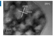
Zeolite's mesoporous cousins: High-surface-area single-crystal-like anatase-TiO<sub>2</sub> was synthesized by a simple solution-growth method. This method produces a controllable mesoporous network and preferential exposure of the highly active (001) planes (see TEM) and is readily extendable to the synthesis of other mesoporous single crystals for application in, for example, catalysis and energy storage.
