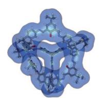
Molecular solids go porous: An imine-linked organic cage exhibits exceptional surface area ( $SA_{BET} = 1375 \text{ m}^2\text{ g}^{-1}$ ) and selective gas sorption, suggesting that porous molecular organic solids could compete in the future with porous networks such as polymers and metalorganic frameworks.
