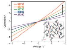
Down to the wire: A simple vapor-transport process using linear diphenylalanine as the starting material has resulted in the self-assembly of cyclodipeptide nanowires with an orthorhombic symmetry. Furthermore, the single-crystalline nanowires exhibit a strong blue luminescence centered at 465 nm and possess semiconducting properties (see picture).
